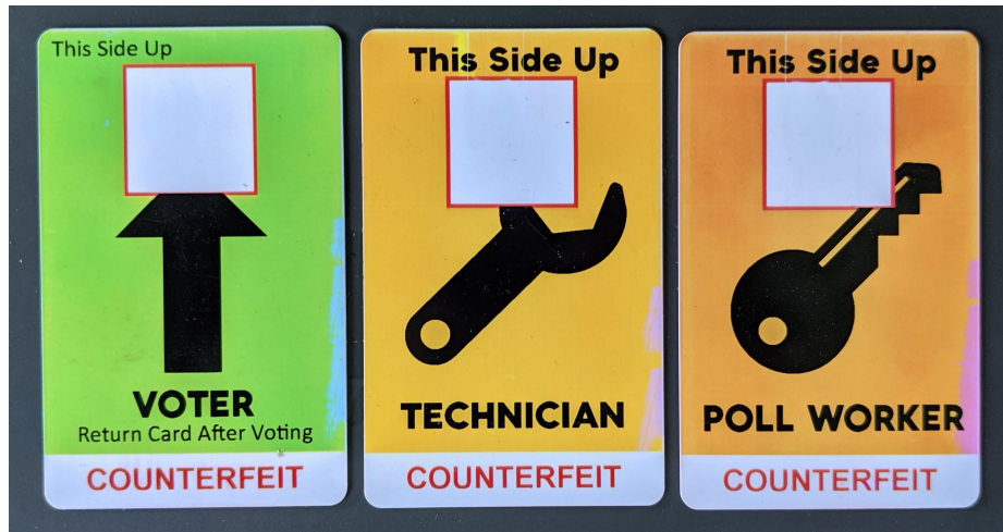
Figure 6: Forged ICX Smart Cards. Weaknesses in the ICX authentication protocol allow an attacker to read and forge Voter, Technician, and Poll Worker cards. I added explicit markings and allowed minor discolorations to minimize any risk of misuse, but a real attacker could create nearly indistinguishable counterfeits.
